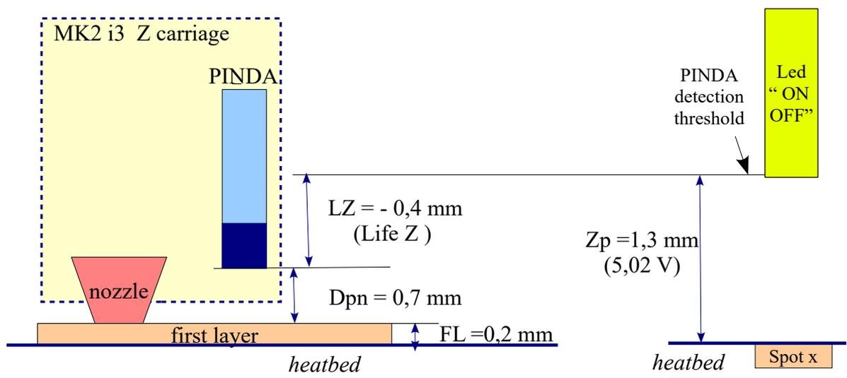
One can presents these results this way , with in mind that the Life Z values are indicative : if I have a PINDA probe with a sensitivity such that it triggers around 1,1 mm and I want to have a distance between nozzle tip and Pinda lowest face of 0,7 mm ( credit card), the Life Z value will be close to LZ # -0,2 mm
